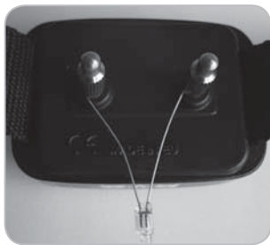
Test discharge lamp connection
