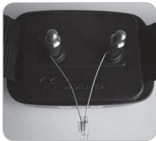
Test discharge lamp connection
