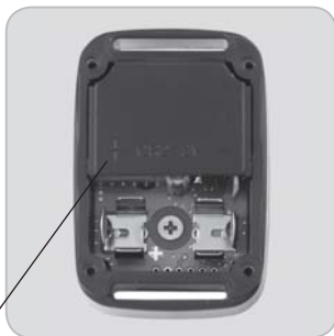
Battery polarity indicator
