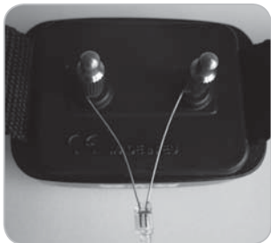
Test discharge lamp connection
